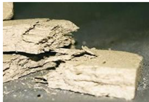
Pieces of Asbestos Insulating Board (AIB)
