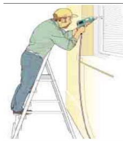
Correct – steps facing work activity
